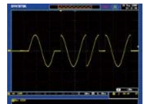
Instantaneous Power Failure
