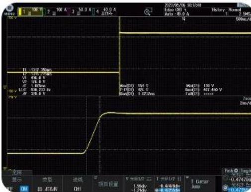
Voltage slew rate of 300V/ms
