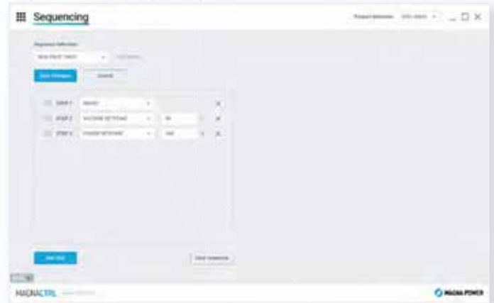
Sequencing Panel Build your own sequence to create operating profiles without writing any code. Add steps from available commands, plus additional commands like time period, abort, and loop commands. When complete, the sequence gets uploaded to the product and stored in memory; no computer connection required after initial programming. PHASE 2 FEATURE RELEASE
