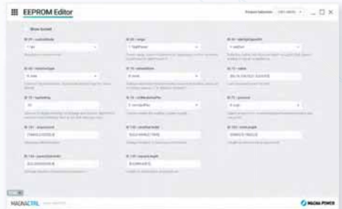
EEPROM Editor Panel Allow Magna-Power applications and support technicians to look behind-the-scenes at the product's configuration parameters using the EEPROM Editor.
