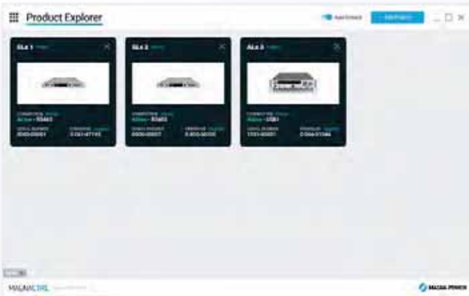
Product Explorer Panel Easily detect connected products and add them to the Product Explorer to make them accessible in the various MagnaCTRL panels. MagnaCTRL retains the product connection details for future sessions, with the ability Auto Connect when the products are detected.
