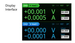
Voltmeter Displays the output voltage with up to 5 digits of Indicators resolution. The default units are Volts (V).
