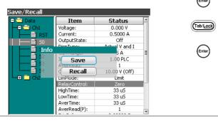
Power-onIn the System Setting menu, the interfaceSettingsparameter settings area shows PowOnSetupsettings. There are 11 settings to choose from, Rst,SAV0~SAV4 and SAV5~SAV9.
