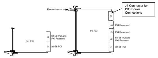
Figure 2-12: 3U and 6U PXI Boards
