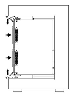
Figure 3-6: Ejector handles position after module insertion
