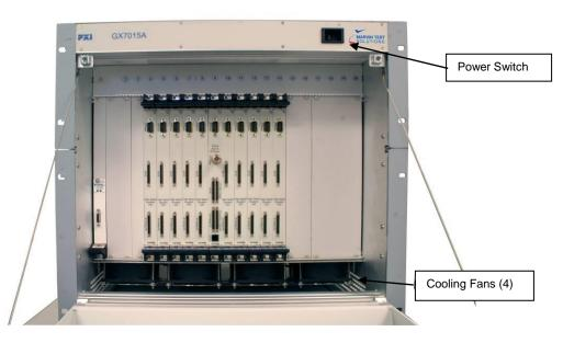
Figure 2-9: GX7015A Front View (configured with GX5960 modules)
