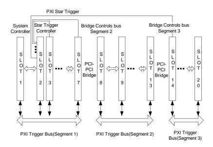
Figure 2-14: PXI Trigger Architecture
