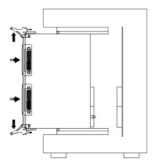
Figure 3-5: Ejector handles position during module insertion
