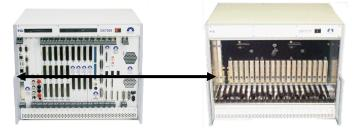
Figure 3-3: Remote configuration with another PXI
