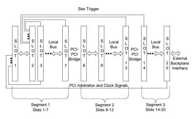
Figure 2-13: PXI Local Bus Routing
