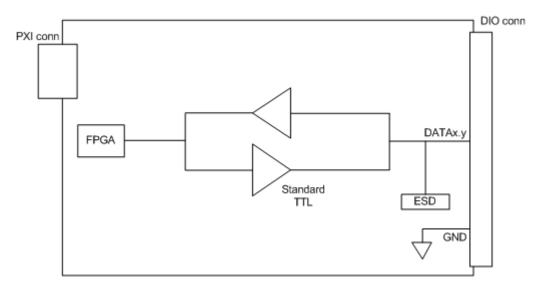
FIGURE 2-8: EMX-7511 BLOCK DIAGRAM
