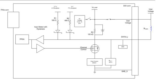
FIGURE 2-6: SINKING CURRENT TYPICAL CONNECTION
