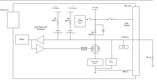
FIGURE 2-5: TTL/LV EMULATION SOURCING CURRENT TYPICAL CONNECTION
